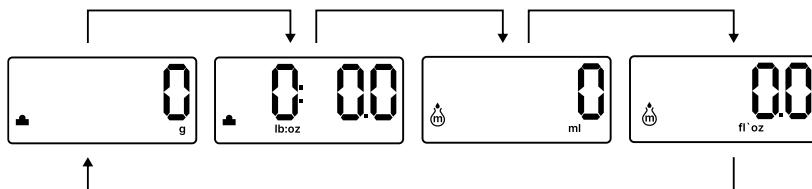
When either milliliters of milk or fluid ounces of milk is selected – there will be an 'M' symbol present on an LCD display.
